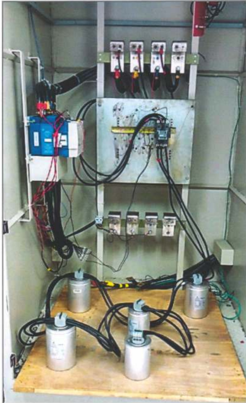
Test set up Photo for 25 KVAR Capacitor Duty Contactor
