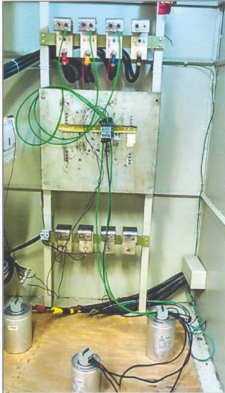
Test set up Photo for 12.5KVAR Capacitor Duty Contactor
